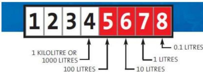
The current reading on this meter is 1,234 kilolitres plus 567.8 litres or 1,234.5678 kilolitres.
